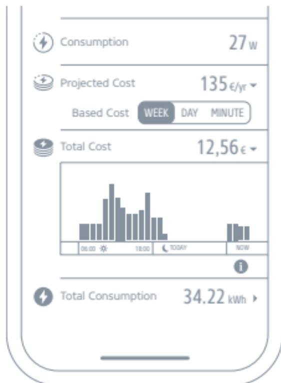
Projected cost can be calculated based on the consumption of the last minute, day or week. Go to Settings > General > Energy Cost to enter your electricity rate and accurately calculate costs.
