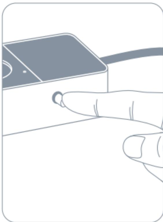
If an electrical surge is detected, the fuse on the side of Eve Energy Strip will eject and the protection indicator LED will turn off.
